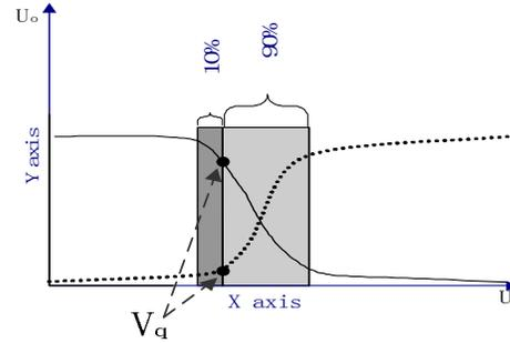
**Figure 4. Input-Output feature of a transistor**
