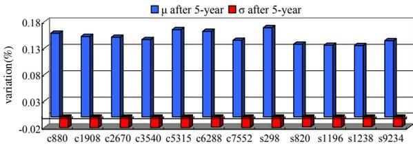
Figure 3. Circuit delay distribution under PV and aging effects.
