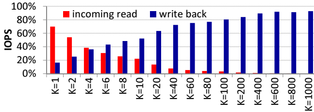
Figure 14: Opportunity study for serving incoming reads while flushing buffered writes as in the flushing algorithm in Figure 4.
